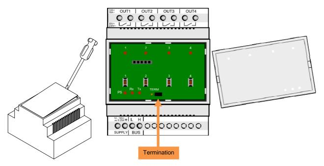
Generally, only 2 'TERM' terminators must be used in a complete Velbus<sup>®</sup> installation. Usually, this will be on one module inside the distribution box and on the module which is physically located furthest from the distribution box.
