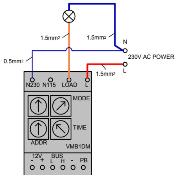
**Warning:** Place the 'mode' rotary switch on one of the following positions: 0, 1, 2, 3, 4, 5, 6 or 7.
