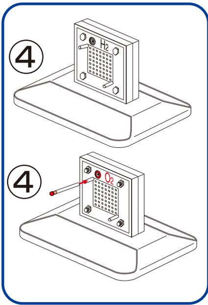
**4.** Insert the reversible fuel cell, terminals on top, into the slot on the base. Cut 2 x 4cm length pieces of rubber tube and insert a black pin into the end of one tube. Place the tube with the black pin into the top pin on the hydrogen side (with black terminal). Place the other tube firmly onto the top input nozzle on the oxygen side.
