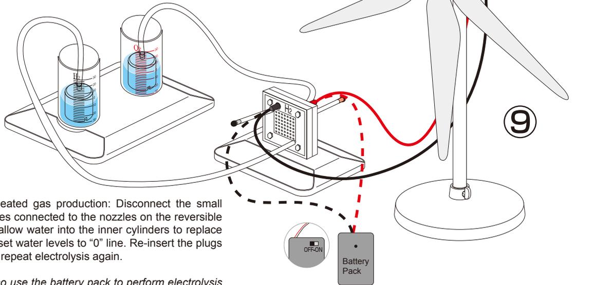
Procedure for repeated gas production: Disconnect the small plugs from the tubes connected to the nozzles on the reversible fuel cell. This will allow water into the inner cylinders to replace the gasses and reset water levels to "0" line. Re-insert the plugs into the tubes and repeat electrolysis again.
