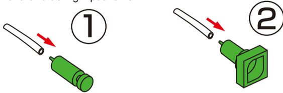
*TIP: To fit the flexible tubes onto the nozzle of the valve, connect the tube by twisting it against the nozzle, then push the nozzle into the tube until the tube is snugly fitted to the base of the nozzle.*
