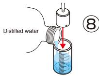
Procedure for repeated gas production: Disconnect the small plugs from the tubes connected to the nozzles on the reversible fuel cell. This will allow water into the inner cylinders to replace the gasses and reset water levels to "0" line. Re-insert the plugs into the tubes and repeat electrolysis again.
