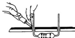
2- Make sure the solder joints are cone-shaped and shiny
