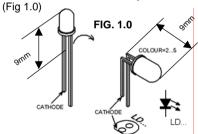
Next: Mount this LED like in the drawing (fig. 2.0). Solder one lead, check the position, if necessary correct it by heating the soldering. Last solder the second connection.
