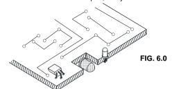
Make sure the transistor connections do not contact any other parts of the circuit.
