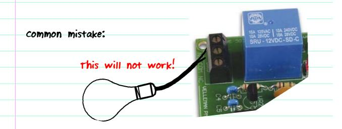
Remember: Relay outputs are switches i.e. There is No voltage coming out of them. You have to apply an external source.
