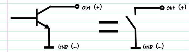
Example: How to switch an LED by means of an open collector output
