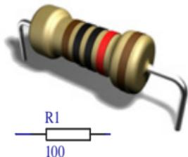
Various **resistor** values are supplied. They serve as current limiters or as voltage dividers. Resistors do not have a polarity. Resistors values are indicated by means of coloured rings. The unit of resistance is called 'Ohm'. ( see colour code table in the package)
