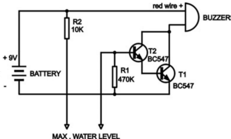
T1 & T2 are configured as a Darlington switch hence only a very small current is needed to make T1 conduct and activate the alarm sound.
