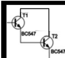
In electronics, the Darlington circuit is a structure consisting of two bipolar transistors connected in such a way that the current amplified by the first transistor is amplified further by the second one. This configuration gives a much higher current gain than each transistor taken separately.
