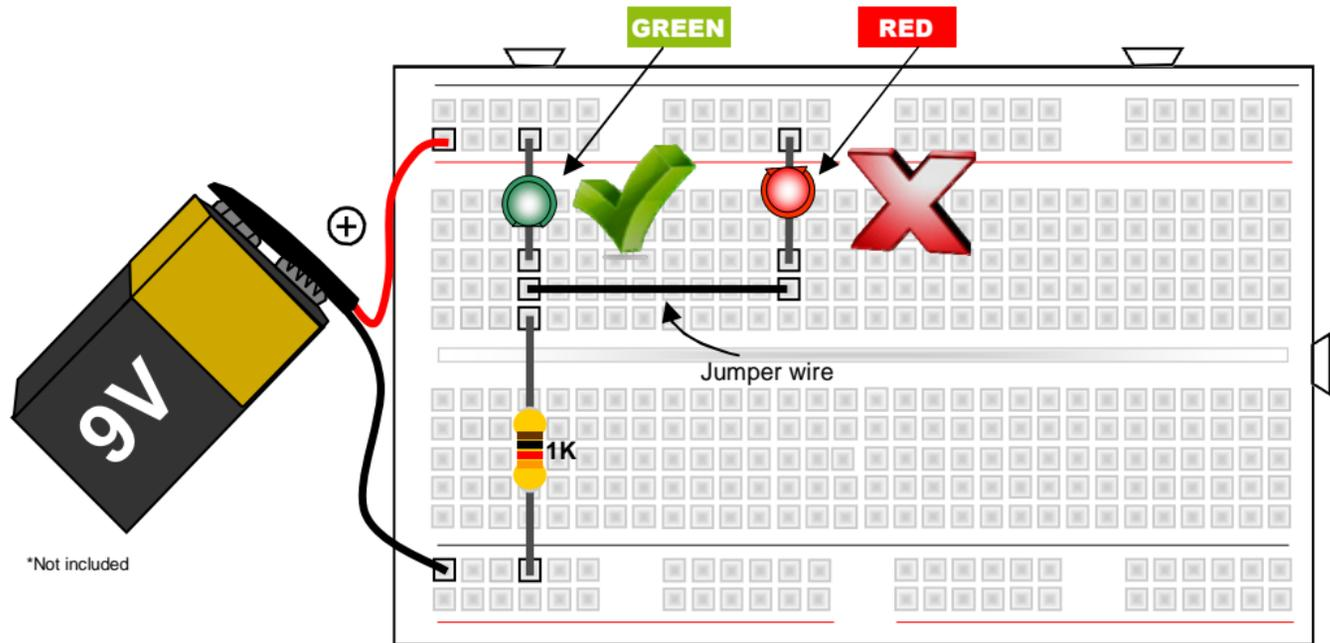
**Required parts:** 9V battery\*, 1K resistor (brown black red gold), red LED, green LED, wire jumper
