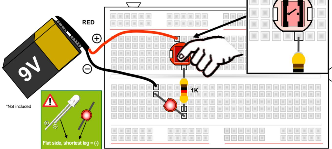
**Required parts:** 9V battery\*, 1000 ohm resistor (brown black red ), red LED, push-button
