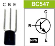
A transistor is an amplification device. By means of a small current, a much larger current is controlled. Transistors come in two flavours, NPN and PNP-types, depending on the polarity. With this kit, you receive a BC557 (PNP) and a BC547 (NPN) transistor. A transistor has 3 pins: Base, Emitter and Collector.
