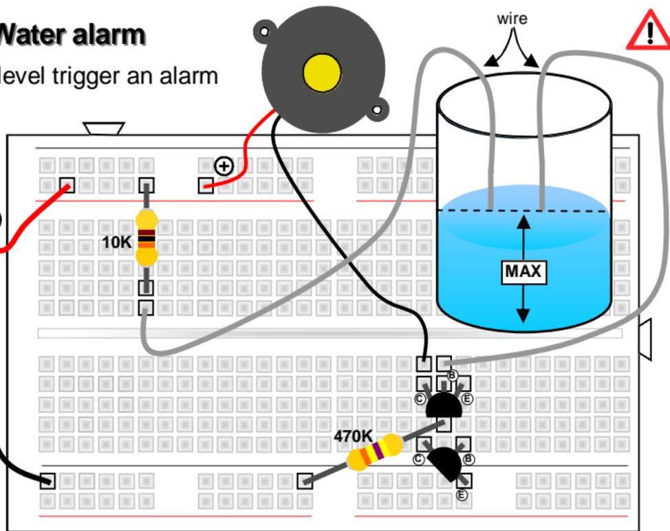
**Required parts:** 9V battery, 10K resistor (brown black orange gold), 470K resistor (yellow purple yellow gold), buzzer, 2x BC547 transistor, 2 wires
