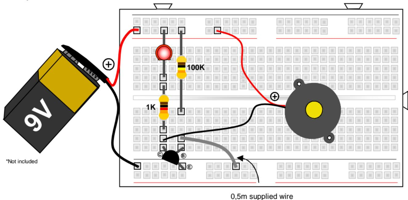
**Required parts:** 9V battery\*, 1K resistor (brown black red gold), 100K resistor (brown black yellow gold), red LED, BC547 transistor, buzzer, 0,5m supplied wire.
