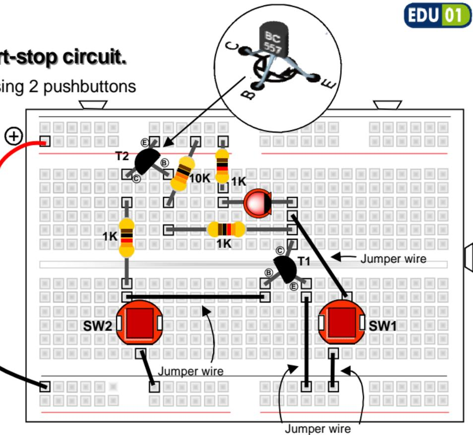
**Required parts:** 9V battery\*, 3 x 1K resistor (brown black red gold), 10K resistor (brown black orange gold), red LED, 2 x push-button, 1x BC547 transistor, 1x BC557 transistor, 5 x wire jumper
