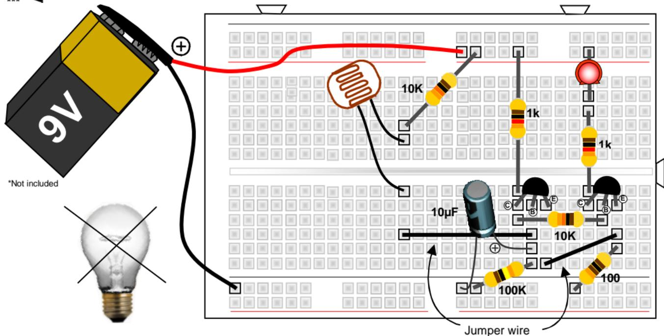
**Required parts:** 9V battery\*, 100 ohm resistor (brown black brown gold), 2 x 1K resistor (brown black red gold), 2 x 10K resistor (brown black orange gold), 100K resistor (brown black yellow gold), 2x BC547 transistor, 10 $\mu$ F electrolyte capacitor, LDR, Red LED, 2x wire jumper
